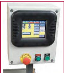
Touch Screen Control Panel
