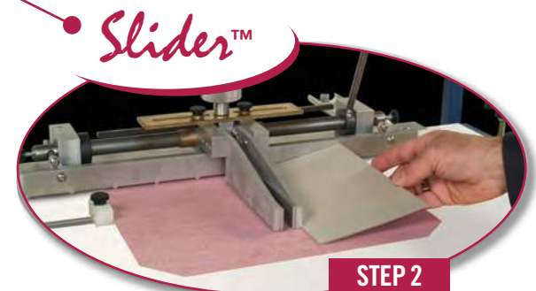
STEP 2 Spots and aligns hard cover boards in position with sliding table case gauge.
