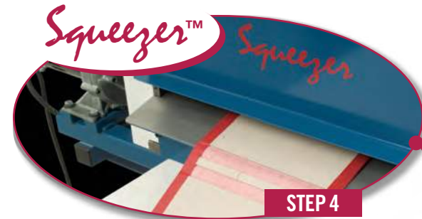
STEP 4 Finished hard cover goes through the rotary press.
