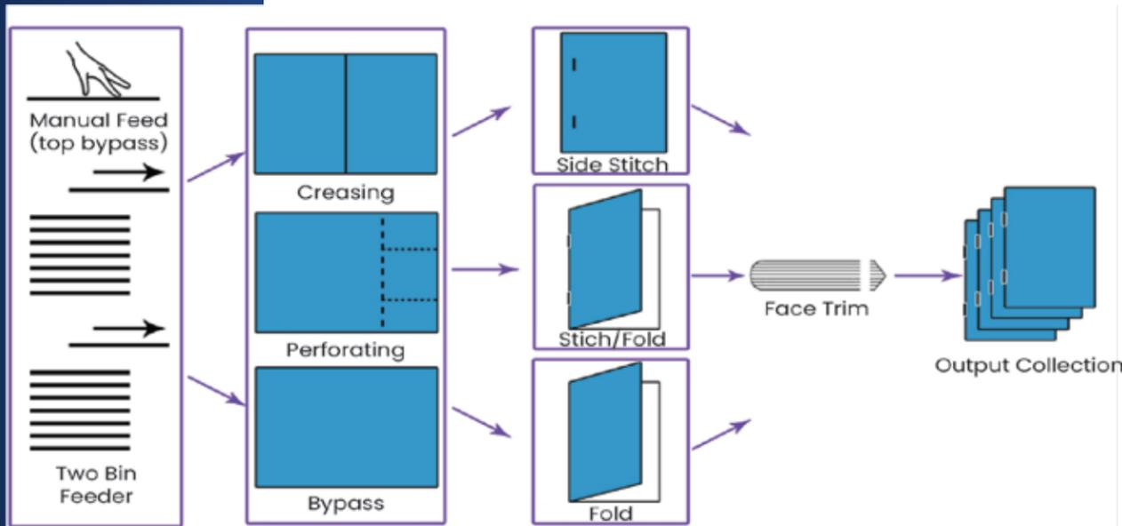
Choose between manual feeding through the bypass or using the dual stage feeding system. Next, add in creasing or perforating through the feeder into the stitch/fold unit. Automatic center alignment, side guide adjustment, and back guide adjustment with jogging make setup inside the machine a breeze with no manual intervention required. Finally, finish strong with programmable trim length adjustment and automatic outfeed roller alignment to retrieve expertly finished booklets.
