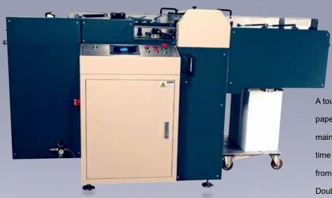
Punching tabs is no problem with the tab jogging option. Signatures and heavy board stock can also be punched with the suction feeder option. No problem changing preselected speeds from the touch screen!
