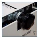
NIPPER CONTROL Controls the height of the nipper. The dwell time can be set up to 3 seconds.
