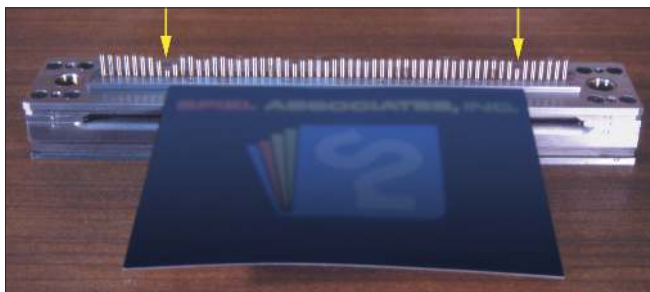
Above, pulled pins are used to ensure a proper margin. Below, unpulled pins result in a questionable margin.
