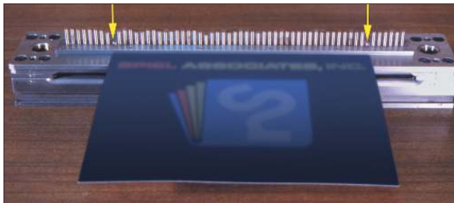
Above, pulled pins are used to ensure a proper margin. Below, unpulled pins result in a questionable margin.
