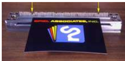
Pins pulled (above) and unpulled (below).
